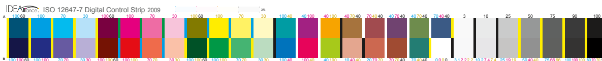
IDEAlliance ISO 12647-7 Color Control Wedge 2009 printed on every Printing Concepts contract proof to ensure consistency.
